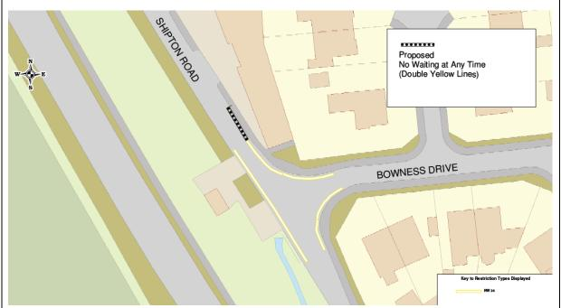
An extension of 10m was recommended to improve forward visibility on approaching the bend/junction.
